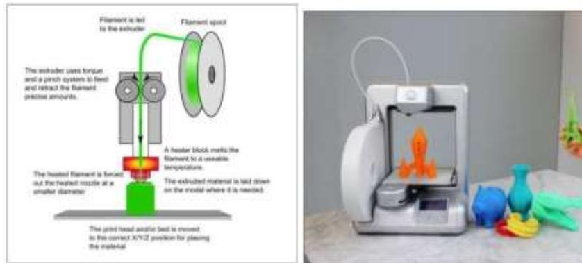
Figure 6: Fused deposition modelling (FDM)
