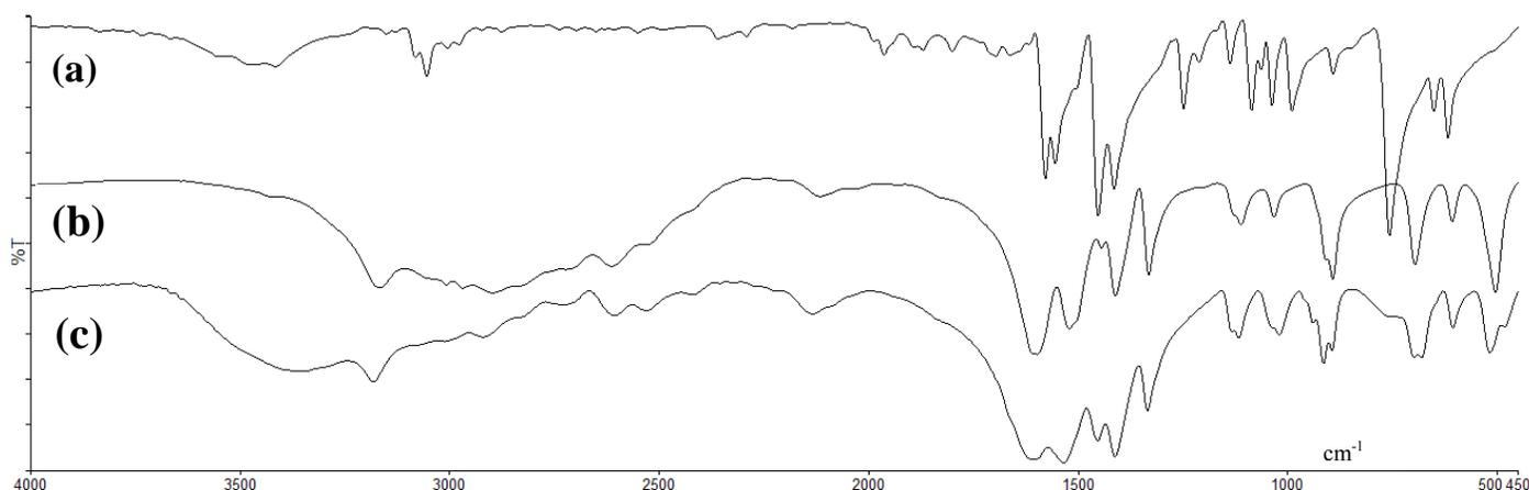
**Fig. 2:** IR spectra of *bipy* (a), glycine (b) and Sm(*bipy*)(*glycine*)<sub>3</sub> (c).
